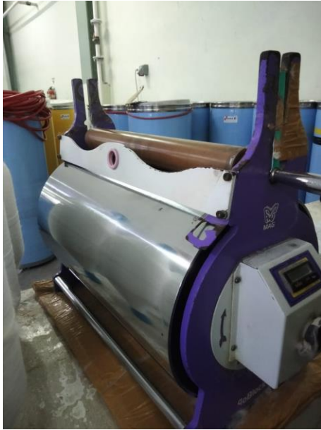
Lampiran 1 Mesin reeling manual
