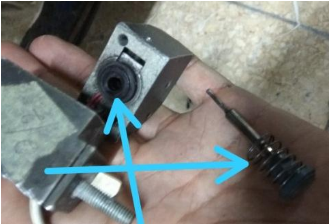
Lampiran 2 seal dan spring di FDP Pin
