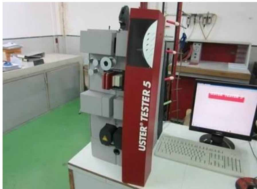
Lampiran 2 Alat Uji Uster Tester 5
