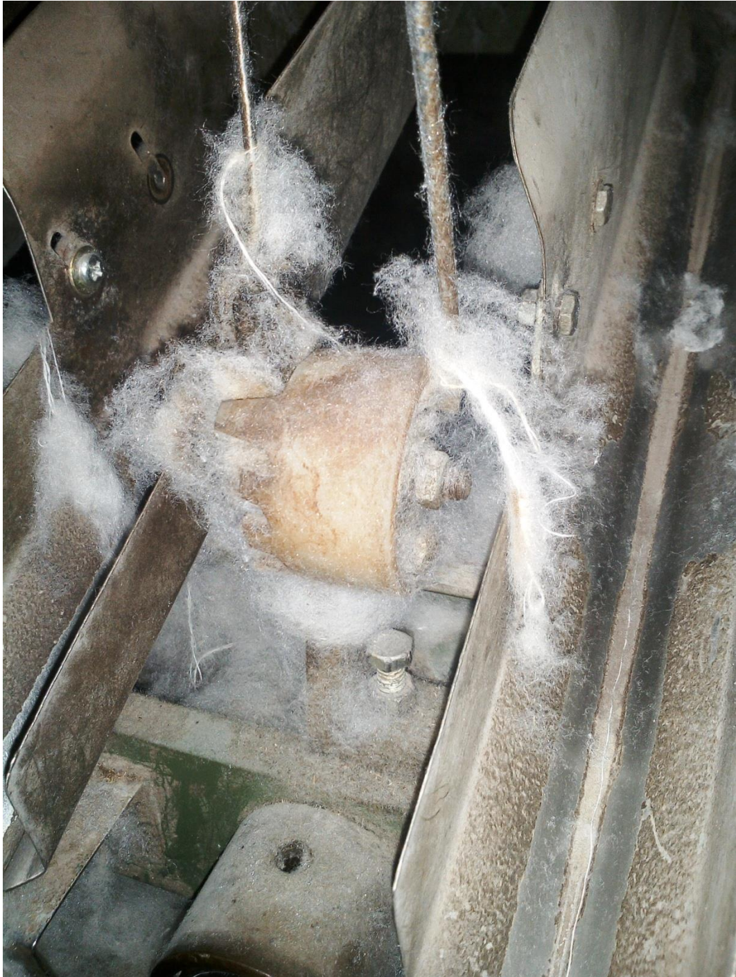
Lampiran 7 Kondisi peer tension kotor
