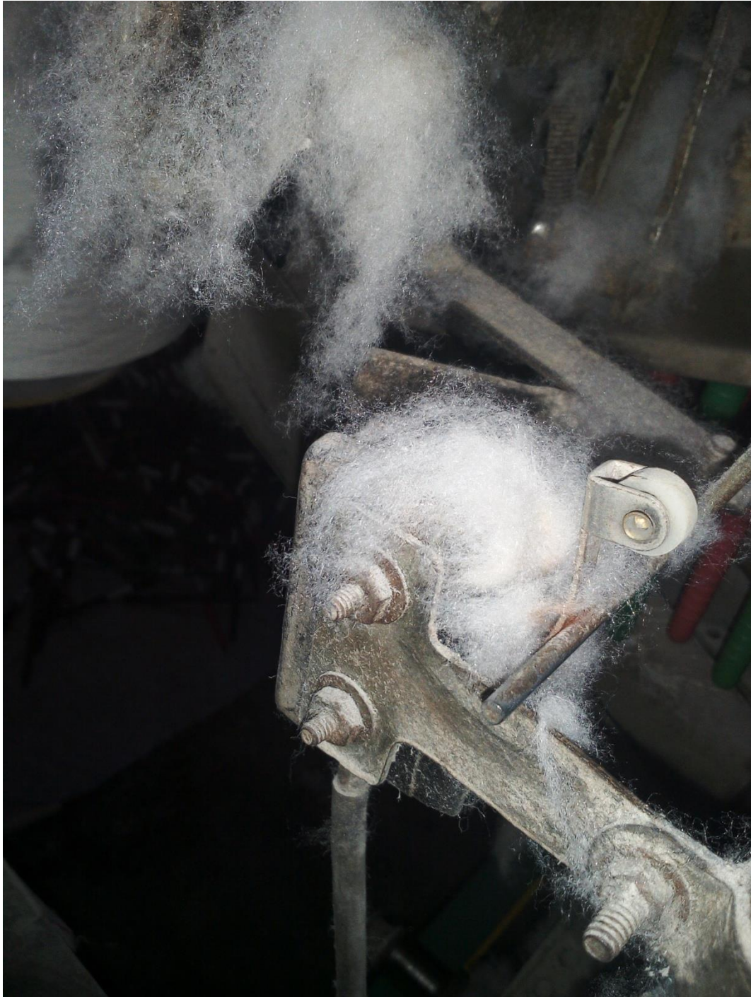
Lampiran 3 Kondisi stop motion kotor
