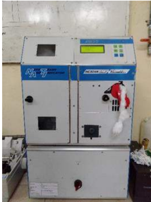
Lampiran 10 Gambar Alat Uji Neps and Trash (NATI)
